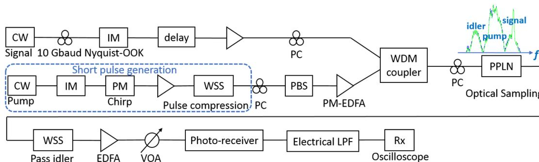
Fig. 2. N-OOK receiver with optical pre-sampling (a) experimental setup (b) simulation setup. CW: constant wave. IM: intensity modulator. PM: phase modulator. EDFA: erbium-doped fiber amplifier. PM-EDFA: polarization maintaining erbium-doped fiber amplifier. WSS: wavelength selective switch. PC: polarization controller. PBS: polarization beam splitter. VOA: variable optical attenuator. LPF: low pass filter. PD: photodiode.
