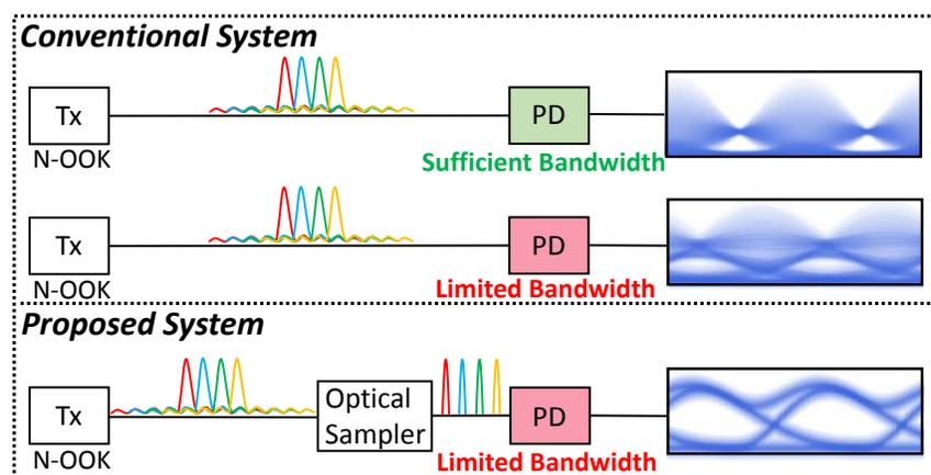
Fig. 1. Principle of band-limited photodiode enhanced by optical pre-sampling.
