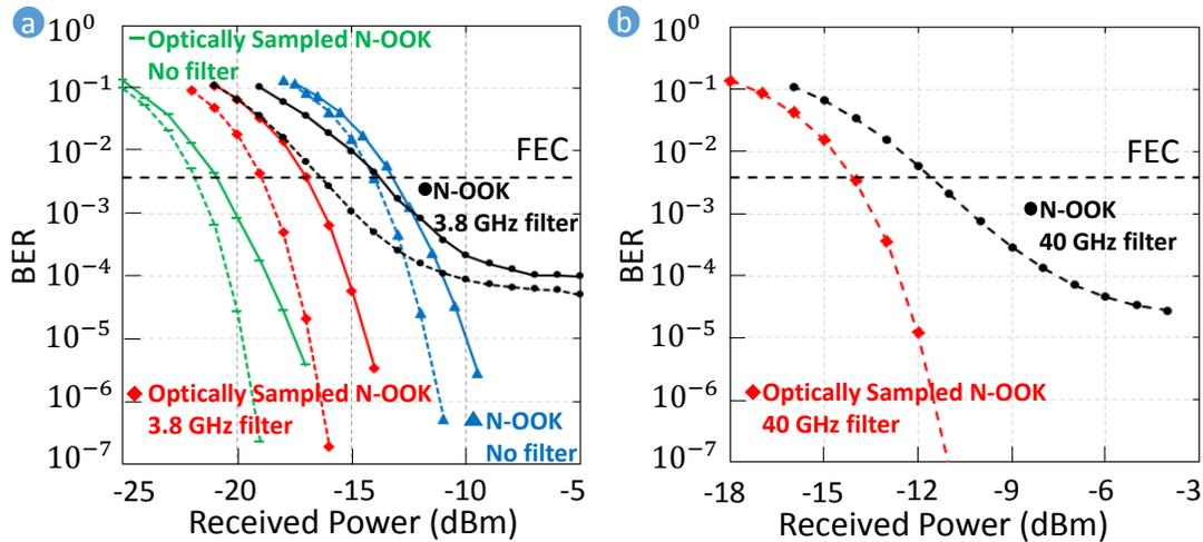
Fig. 3. (a) BER vs. Received Optical Power plot of experiment (solid line) and simulation (dashed line). (b) BER vs. Received Optical Power plot of 100 Gbaud N-OOK received by 40-GHz bandwidth photodiode simulation.
